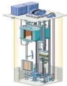
Figure 2.2.1. Passenger Cage Elevator
